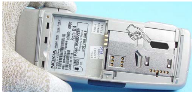
4.) Be sure that the battery is removed and then continue with disassembly. Note to put back the Sealing Tape after the re-assembly.
