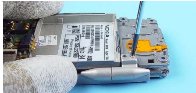
For assembly use a Torx Plus® size 6 driver with a torque setting of 22Ncm.
