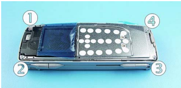
9.) Unscrew the four, Torx Plus ® size 6 screws in the shown order. Always use new screws when re-assembling! For assembly, reverse the order and use a Torx Plus ® size 6 driver with a torque setting of 25Ncm.
