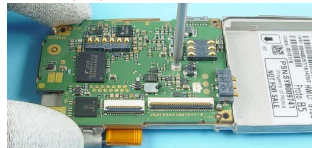
Always use new screw when re-assembling! For assembly use a Torx Plus® size 6 driver with a torque setting of 25Ncm.
