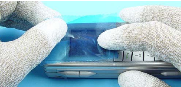
1.) Protect the window with a film.
