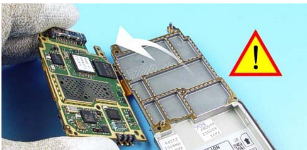
Turn the Engine Module. Take care of the RF Gasket .
