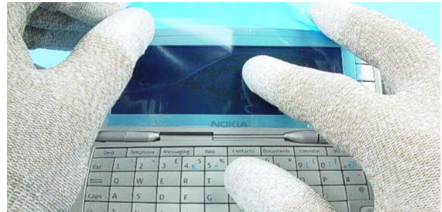
2.) Fit protective film to the LCD Module .
