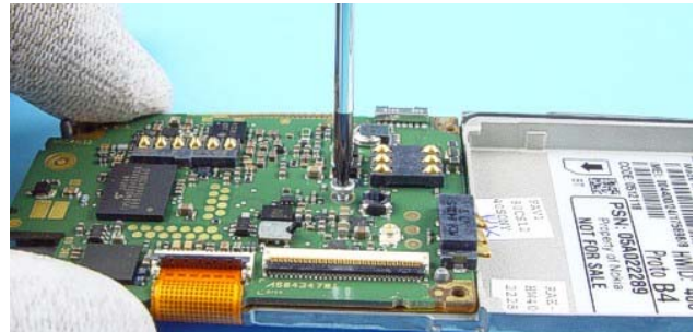
Unscrew the Torx Plus® size 6 screw.
