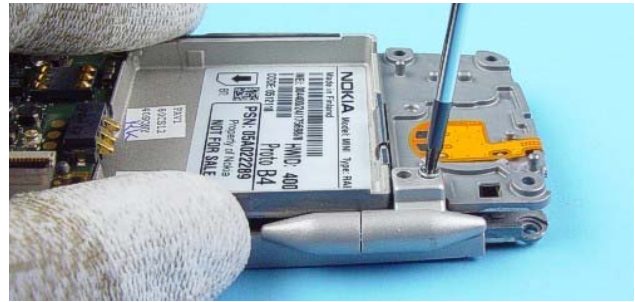
40.) Unscrew the Torx Plus® size 6 screw.
