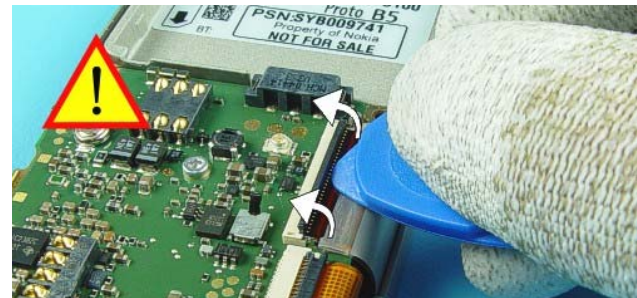
38.) Unlock the flex connector with SRT-6 carefully.
