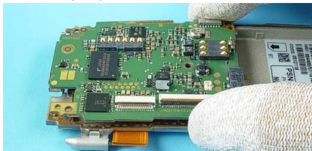
Place the Engine Module onto the Shield . Take care of the RF Gasket .
