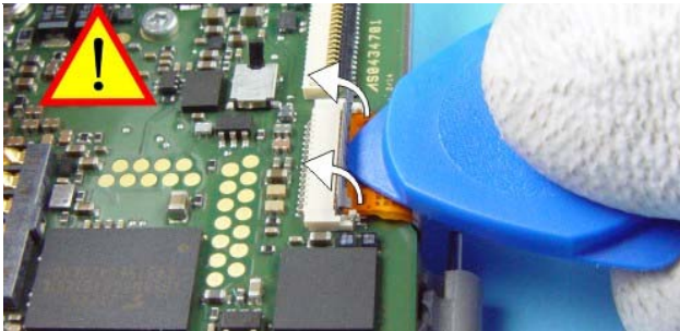
Unlock the connector carefully.
