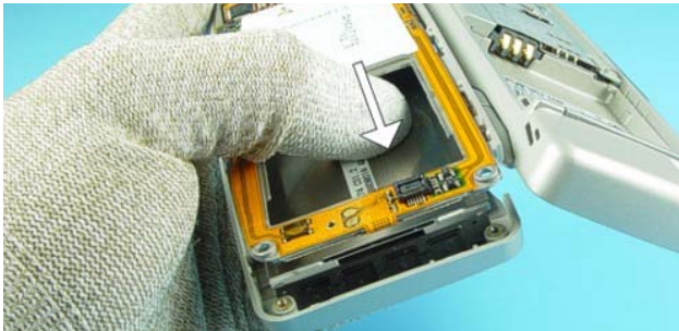
21.) Press out the C-Cover Assy carefully.
