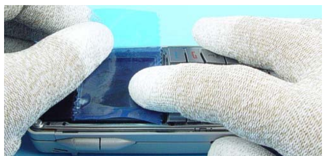
6.) Protect the LCD Module with a film.
