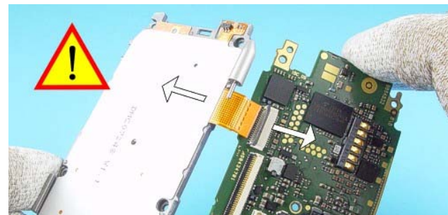
Remove the flex from the connector carefully.
